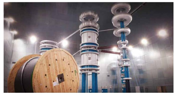
kV test system and 5000 A heating transformer sets. Using a surge generator, we locate potential damage to the cables and wires. In 2021, we completed the expansion of the Laboratory in the R&D Centre, which allowed us extensively research HVDC direct and EHVAC alternating current cable prototypes for higher-rated voltages, and technological guidelines for their production.
