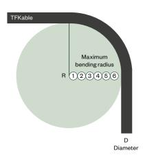
The minimum bending radius describe how tight can be a cable bend without kinking it, damaging it or shortening its lifetime. Minimum bending radius express the smallest possible bend. The smaller the bending radius, the shorter bends you can make. The bending radius is expressed as a multiple of the outer diameter of the cable, for example 6xD, where D is the cable outer diameter.
