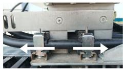
**Figure 3.7**Correct placement of the cable in drag chain
